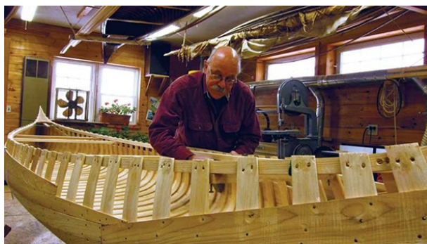
Figure 6. Bruce Larson uses forms that he acquired from the estate of the late Burt Libby for his new canoe construction projects. The ribs and planking are fashioned from white and red cedar. Photo by Roger Moody.
